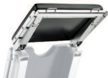
91450 Head rest, standard, tilting up and down with side rails 25 x 10 mm 91453 Head rest, standard, tilting up and down with side rails 30 x 10 mm Standard head rest for the models schaeerer® axis 400 – 700. Length: 400 mm. Continuous adjustment with gas-lift spring assistance.
