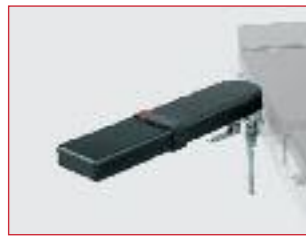
580040 Arm rest Clamp with fixing screw, adjustable up/down and laterally, height adjustable, swivelling through 180°, length 600 mm, width 150 mm 580013 Fixing strap (order 1 piece)
